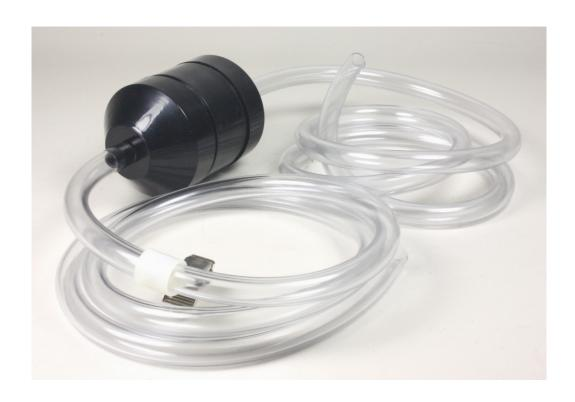
In-line Lapel Filter Holder for Utilization with personal air samplers.
