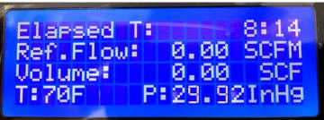
Standard Product (Reporting of flow and volume at ambient conditions of temperature and pressure) **STP OPTION** (Reporting of flow and volume at a Reference temperature and pressure in addition to the reporting at ambient conditions)
