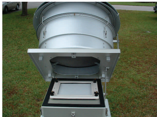
GAS-PM10DE Series System PM10 Inlet Open Position for Access to Filter Paper
