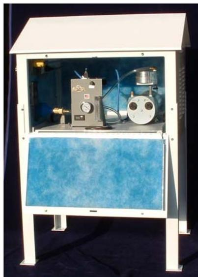
Alternatively, complete packages containing several or all of these components, including the weatherhouse enclosure; have been available from various USA suppliers. Optional items installed in these RETS/REMP air monitoring systems include the items listed in Table B.
